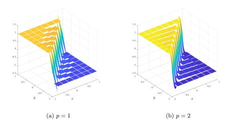
Fig. 14: The interior penalty-best approximation  $\phi^h \in \mathcal{V}^h_{D;p,-1}$  of the smooth step function, with  $n_{\rm el} = 8 \times 8$ , subject to element-wise Gibbs constraints, for different p.
