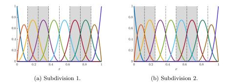
Fig. 11: The two possible subdivisions for  $\mathcal{V}_{2,1}^h$  when  $n_{\rm el} = 8$ . The vertical dashed lines represent the element boundaries.
