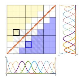
Fig. 16: Subdivision of an  $8 \times 8$  element domain into groups of maximum  $3 \times 3$  elements with approximation space  $\mathcal{V}_{D,2,1}^h$ . The right and bottom inset figures display the univariate basis functions along the corresponding axes.
