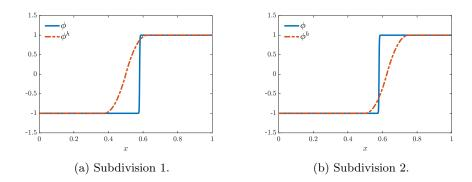
Fig. 12: The  $H_0^1$ -best approximation  $\phi^h \in \mathcal{V}_{D;2,1}^h$ , with  $n_{\rm el} = 8$ , of the smooth step function  $\phi = \phi_{0.58}$ , subject to Gibbs constraints on each of the subdomains illustrated in Figure 11.
